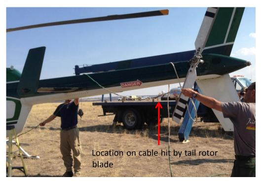
Figure 8. Re-enactment of the cable wrapped around the tailboom.
