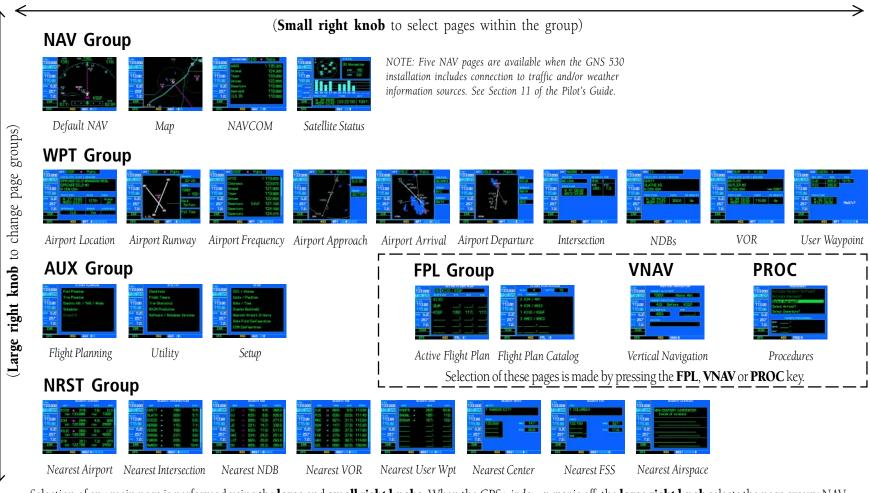
Selection of any main page is performed using the **large** and **small right knobs**. When the *GPS window cursor* is off, the **large right knob** selects the page group: NAV, WPT, AUX or NRST. The **small right knob** selects the desired page within a group. To quickly select the Default NAV Page, press and hold **CLR**.
