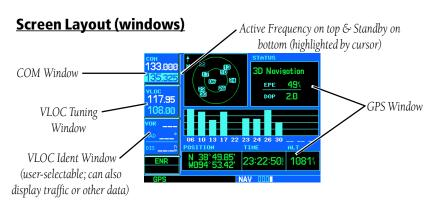
The GNS 530's display is divided into four separate "windows" (or screen areas). The left 1/4 of the display provides a *COM window* (top two lines) and a *VLOC window* (by default with VOR ident/radial, but selectable for other data). The right 3/4 of the display consists of a *GPS window*, which is where you'll find the various navigation, waypoint information and settings "pages". The bottom of the display is used for annunciators.
