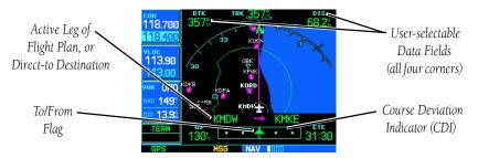
The following symbols are used —directly above the graphic CDI—to depict the "active leg" of a flight plan or direct-to:
