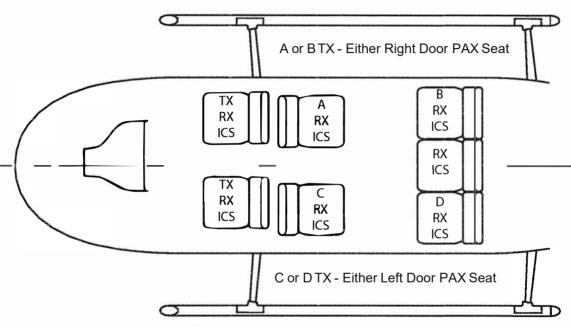
TX - Radio Transmit Capability RX - Radio Receive Capability ICS - Intercom Capability
