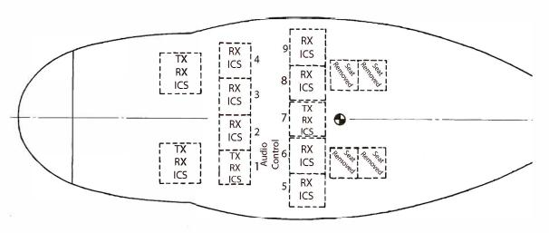
The aft audio control shall face position 6. The Spotter's position is position 7.
