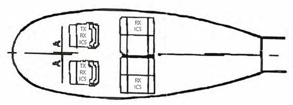
TX - Radio Transmit Capability RX- Radio Receive Capability I CS- Intercom Capability
