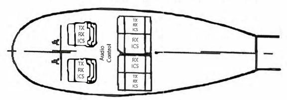
The aft audio control shall be ceiling mounted and face the middle of the two center PAXseats
