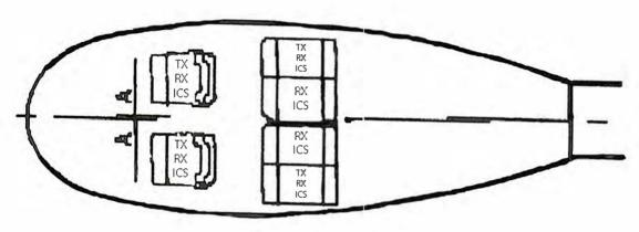
TX - Radio Transmit Capability RX- Radio Receive Capability ICS- Intercom Capability
