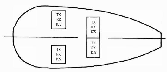
TX - Radio Transmit Capability RX - Radio Receive Capability ICS - Intercom Capability
