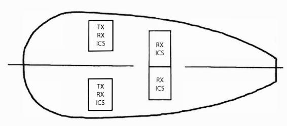
TX -Radio Transmit Capability RX -Radio Receive Capability ICS -Intercom Capability
