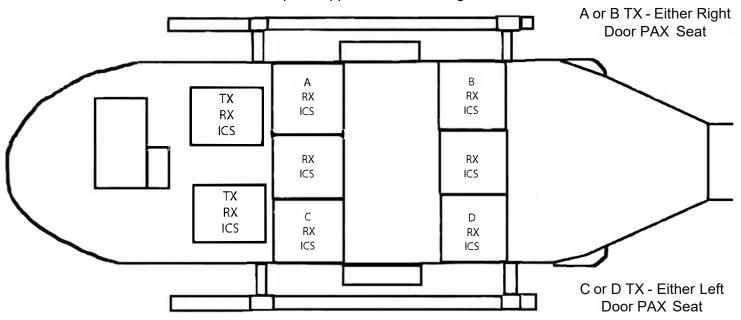
TX - Radio Transmit Capability RX - Radio Receive Capability
