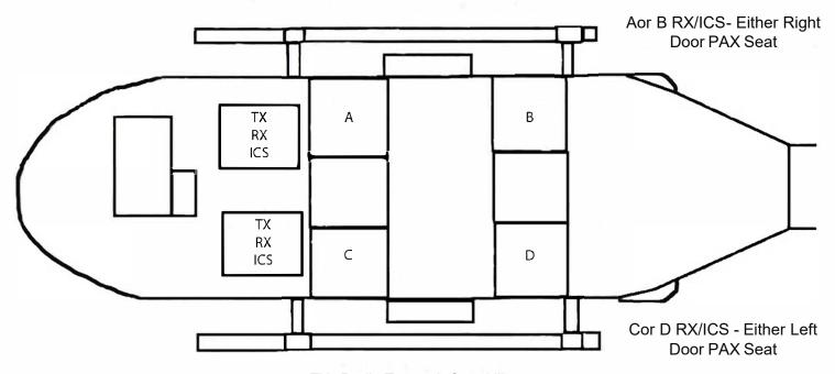
TX- Radio Transmit Capability RX - Radio Receive Capability
