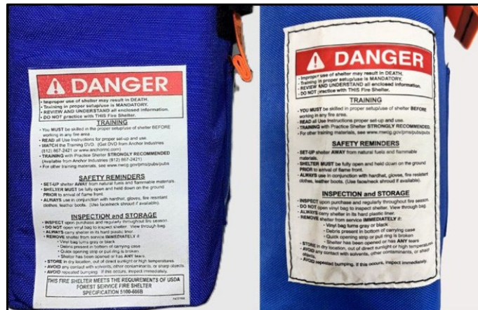
Figure 3: Left is a specification carrying case with heat-pressed label, right is a non-specification carrying case with label stitched on.
