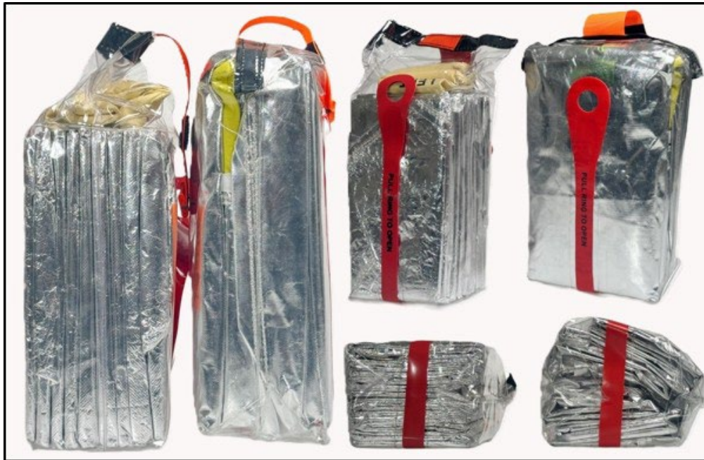
Figure 7: Specification shelters, left in each pair, and non-specification shelters, right in each pair, showing incorrect, sloppy folding and buried shake handles.
