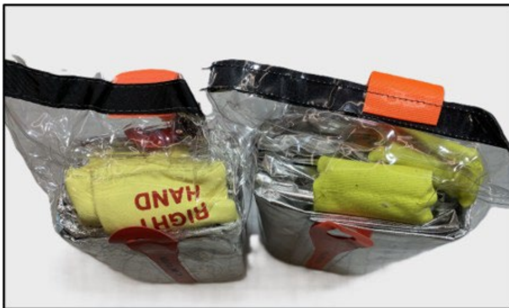
Figure 8: Specification shelter on left, non-specification shelter on right. Note missing stenciling on shake handle on non-specification shelter.
