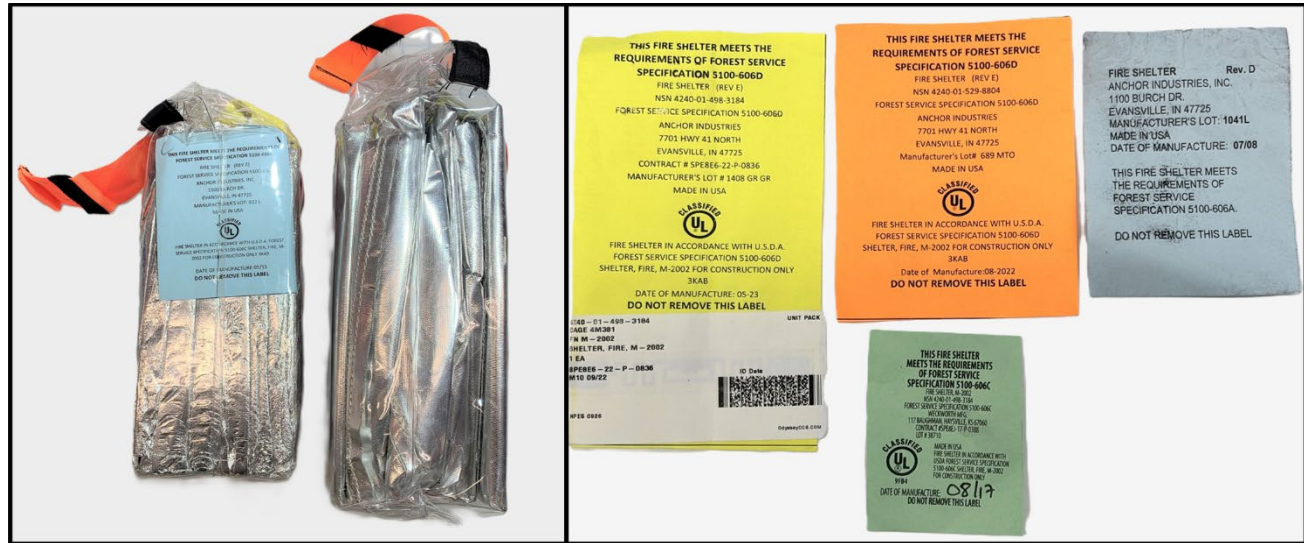
Figure 6: Left image shows missing insert label on non-specification shelter. Right image shows different specification label sizes and colors.
