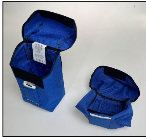
Figure 4: Specification carrying case on left, non-specification on right. Note the non-specification case is missing the label and is unable to stand on its own.
