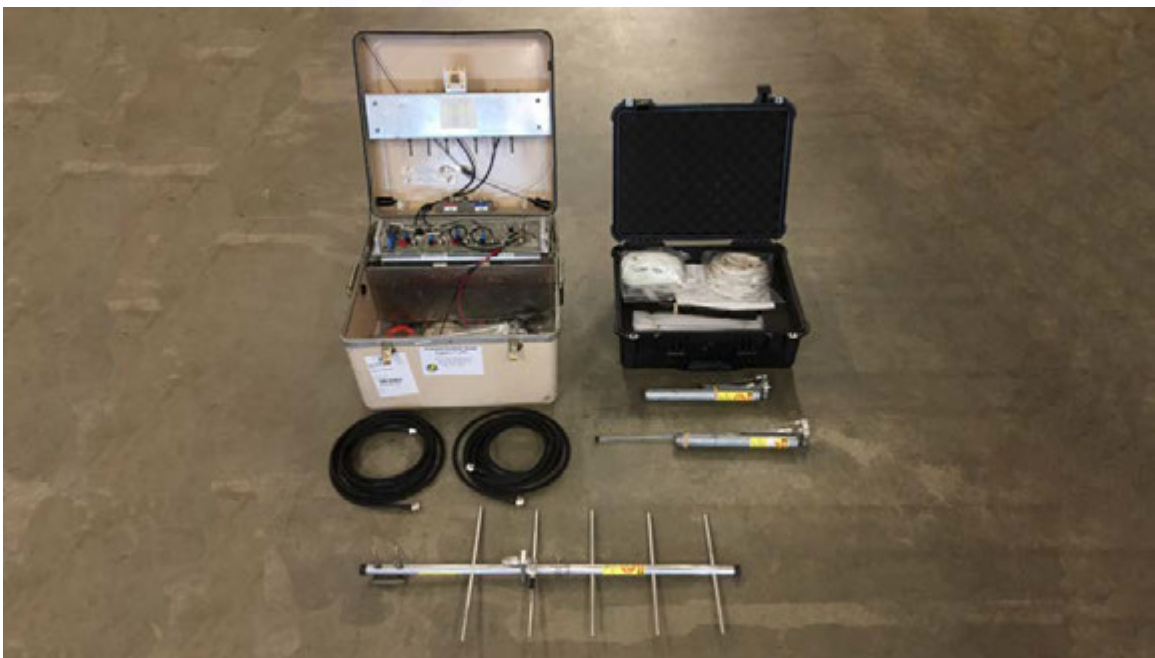
NFES# 004312 VHF Command Repeater/Link Kit w/ NFES# 004100 Mountain Top Accessory Kit
