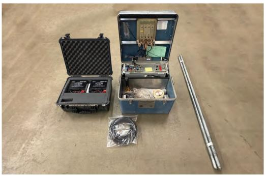
NFES# 004248 UHF Logistics Repeater Kit Components with NFES# 004150 Sealed Lead Acid Battery Kit
