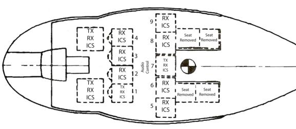
Passenger positions 1 & 7 have TX, RX and ICS capability. All other passenger positions have RX and ICS capability.
