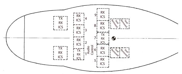
Passenger positions 1 & 7 have TX, RX and ICS capability. All other passenger positions have RX and ICS capability.
