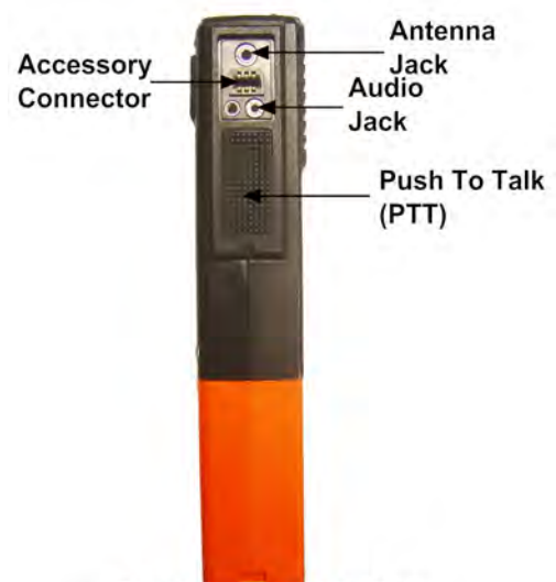
Figure 3: DPH Side View
