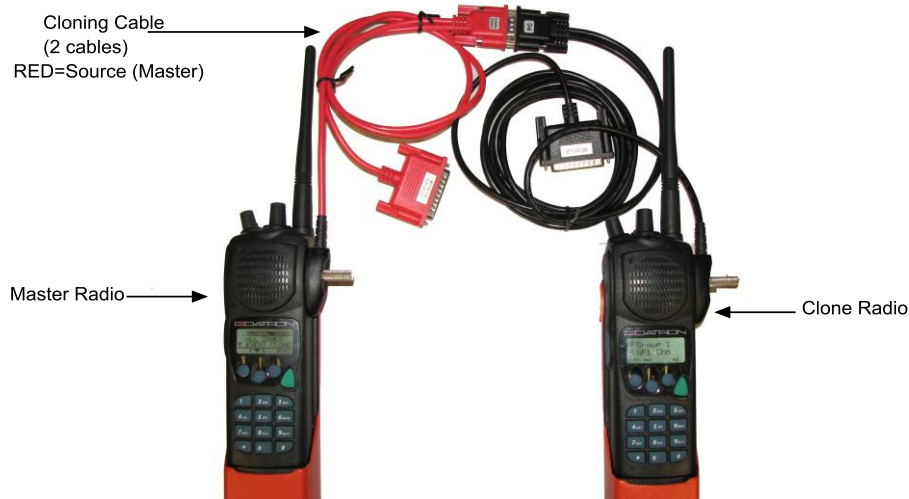
Fig. 8: Cloning Cable Connections
