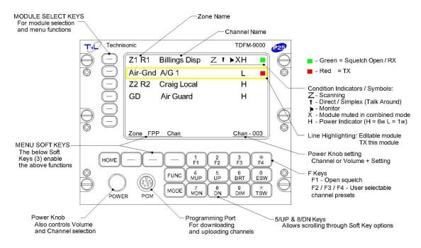
TDFM-9000 series radio buttons have multiple configuration options depending on how they are setup during initial programming using Motorola's CPS software. The NIICD TDFM-9000 Quick Reference Guide only applies to TDFM-9000 radios configured using a NIICD codeplug.
