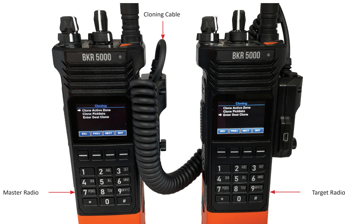
Figure 1: BKR 5000 Cloning Connections
