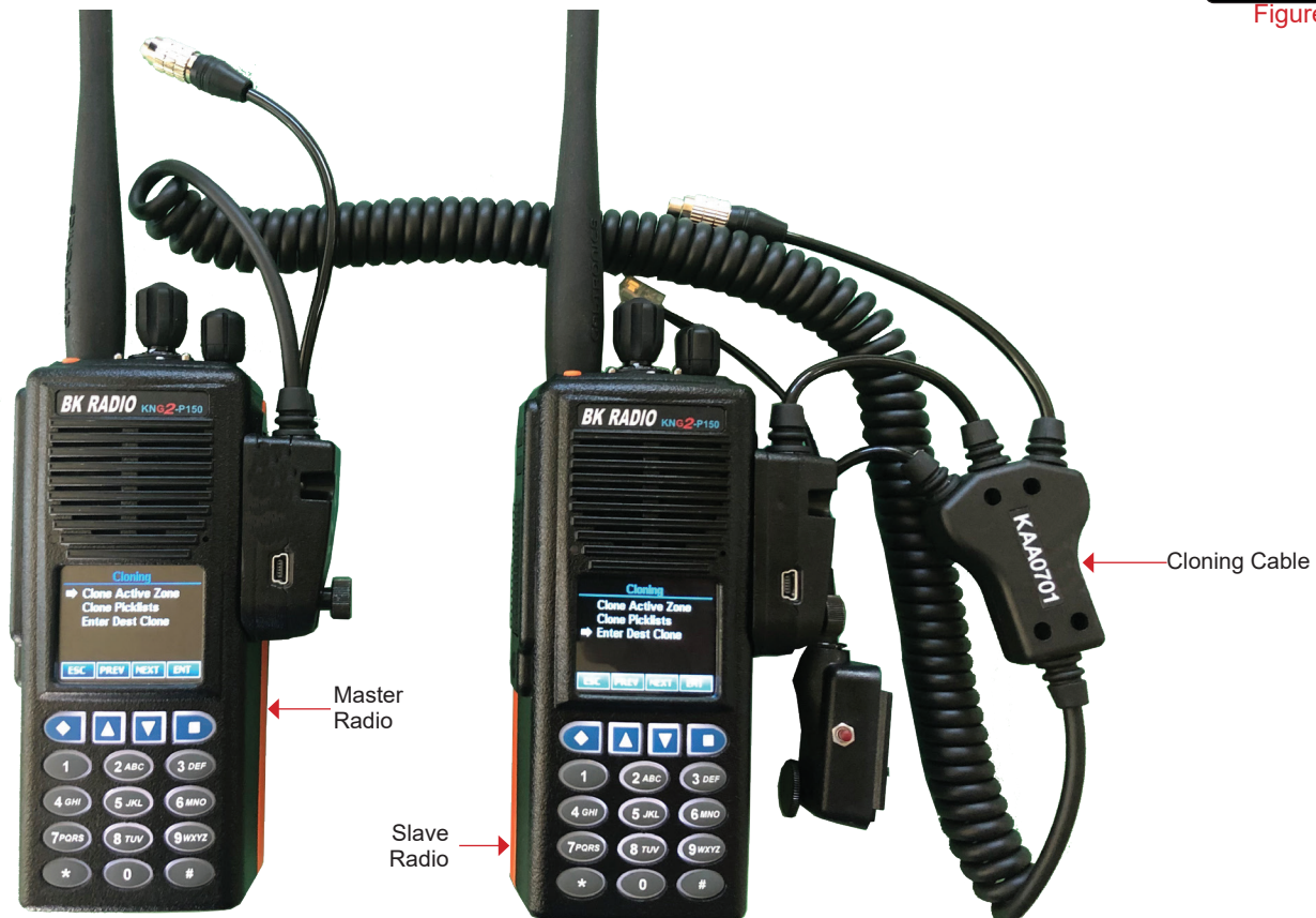
Figure 1 KNG2 Cloning Connections
