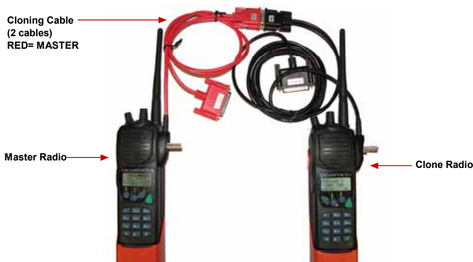
Fig. 8: Cloning Cable Connections
