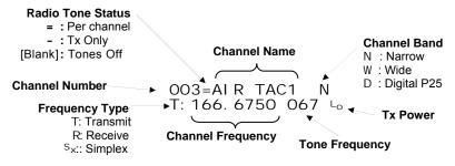
Toggle the **DISP +/-** Switch to view receive or transmit frequency.
