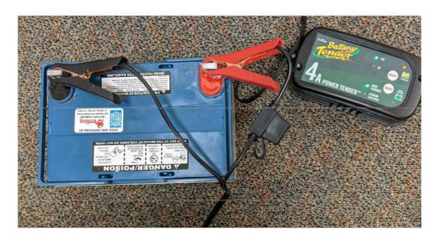
2. Connect charging clips to begin charge. An completely discharged battery will take about 10-hours to fully charge. Battery is charged when indicator light is green.
