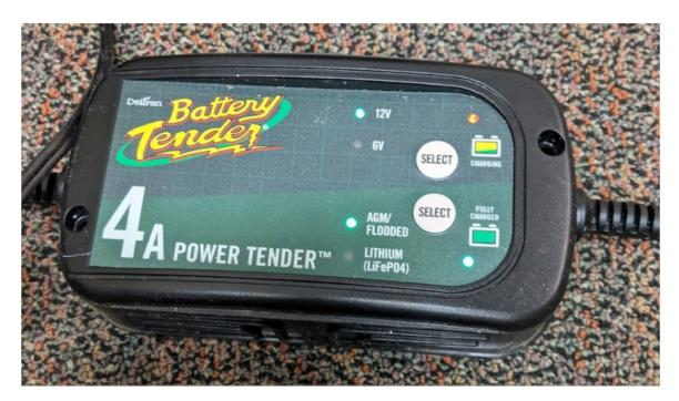
Configure charger for 12V and AGM/Flooded using the select button
