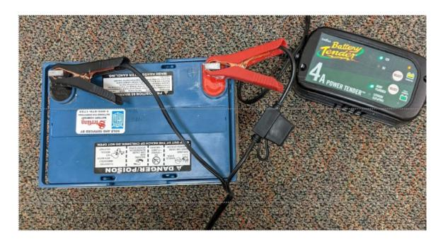
Connect charging clips to begin charge. An completely discharged battery will take about 10-hours to fully charge. Battery is charged when indicator light is green.
