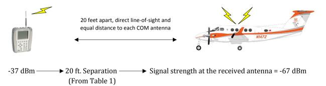
The IFR 4000 is generating a signal on 122.925 MHz and Com 1 is tuned to 122.925 MHz
