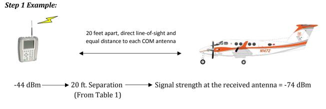
Path loss = 30 dB at 20 feet separation between the IFR 4000 and the aircraft
