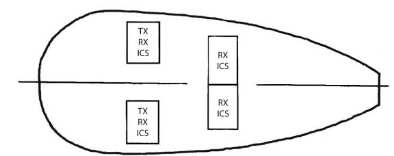
TX - Radio Transmit Capability RX - Radio Receive Capability ICS - Intercommunications Capability
