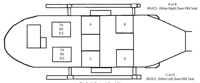
TX - Radio Transmit Capability RX - Radio Receive Capability ICS - Intercommunications Capability
