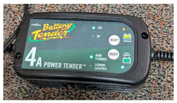
1. Configure charger for 12V and AGM/Flooded using the select buttons
