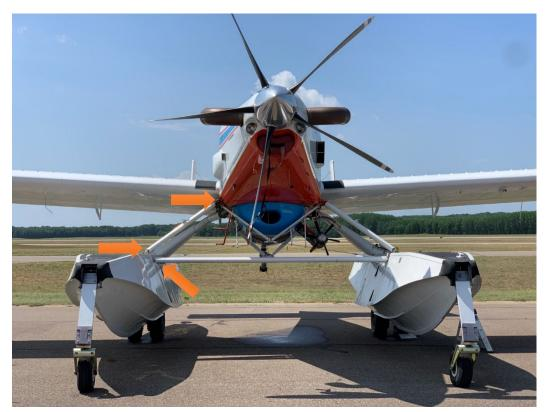
Look at the connecting points on each float for any obvious signs of damage or missing items.
