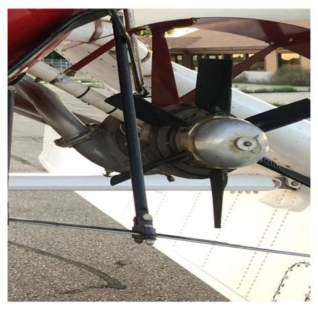
Make sure all blades are attached to prevent any damage.
