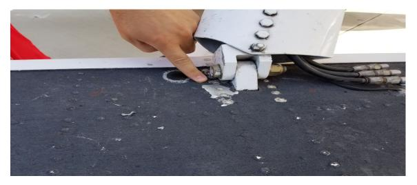
**Cracked or chipped paint around connecting points could be an indication of another issue.** Check with the pilot or crew chief if you see this.
