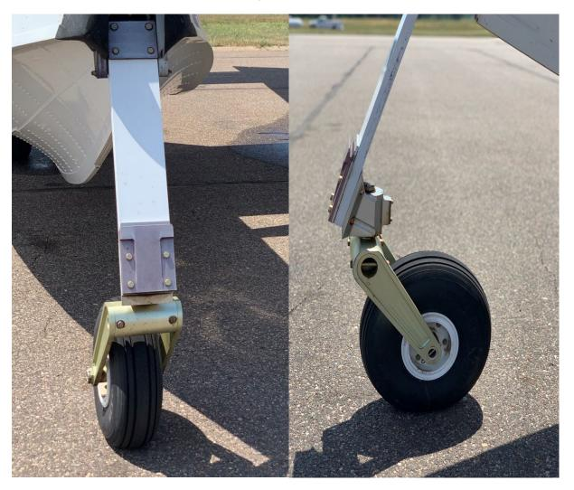
Look for cracks, missing or loose bolts, excessive tire wear and overall good condition.
