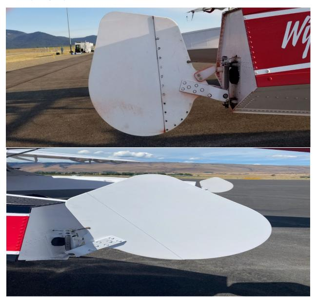
Look at the cable, spring, mounting hardware and rivets for any wear or missing items.
