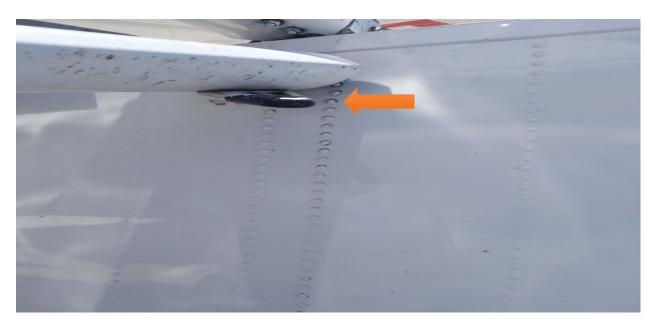
Check for loose or missing rivets. They can be spotted against the white paint scheme.
