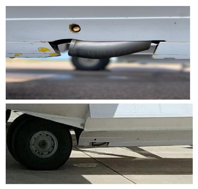
**Look for damage or leaks.** Leaks can be an indication of a bad or loose "Platypus Valve". This valve is a self-closing one way valve that needs flow rate to open.
