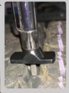
Measure in a main tread groove.
