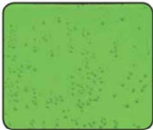
GREEN for conventional low-silicate coolant without SCA
