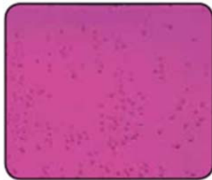
PURPLE/PINK for fully formulated ethylene glycol-based coolant with SCA
