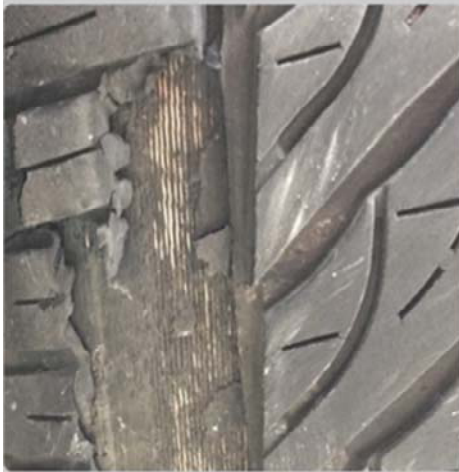
Missing tread blocks (chunking) with cords exposed
