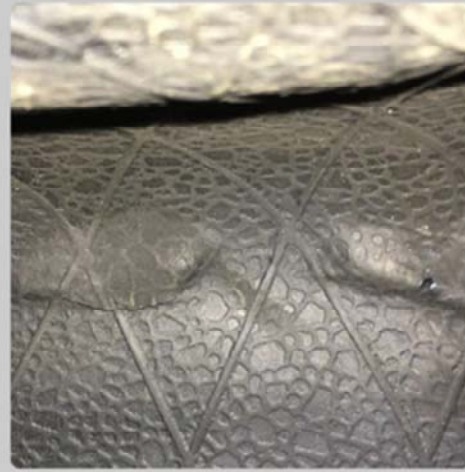
Blister inside the tire from driving on it while it was under inflated
