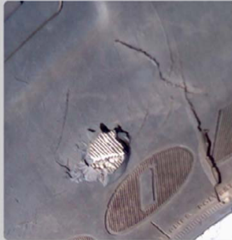
Blister inside the tire from driving on it while it was under inflated
