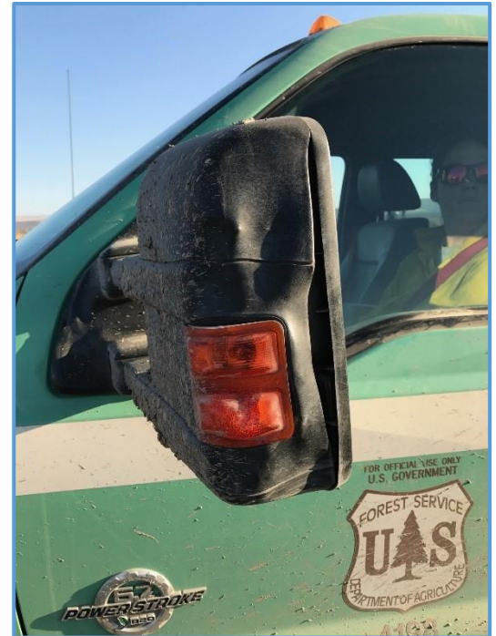
Radiant heat damage to driver's side mirror on E601.
