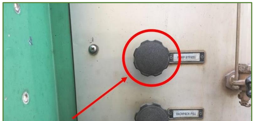
Figure 2 – The location where the Pump Bypass Line enters and exits the valve is behind the control knob on the operator's panel. Disconnect both the entering line and the exiting line. Once the Pump Bypass Line has been disconnected in the described three locations, apply pressurized air from a compressor. The pressurized air should be applied to both the line of the disconnected lines.
