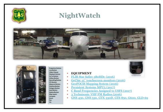
Air Attack 51 is an Air Attack platform based in Southern California on the Angeles National Forest. Even though the primary mission is to provide night aerial supervision, the aircraft is equipped with the same EO/IR capability as the FireWatch Cobra and is able to provide similar over watch and fire mapping support to Fire Managers.
